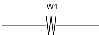
Figure 1.5: W1 element (Warburg impedance, cf. Handbook of Electrochemical Impedance Spectroscopy. Diffusion impedances: http://www.bio-logic.info/potentiostat/notesheis.html ).
